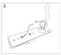
Lay the three-core cable to the track installation site. Connect the protective ground wire to the yellow-green wire on the power lead-in housing. Pull the phase and neutral wires through the hole in the back side of the power lead-in.
