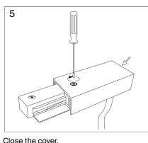
Secure the cover with a screw on the front of power input.
