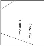
prepare the mounting surface mark and drill the holes insert the dowels into the holes
