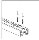
adjust the installation height using the collet fixtures
