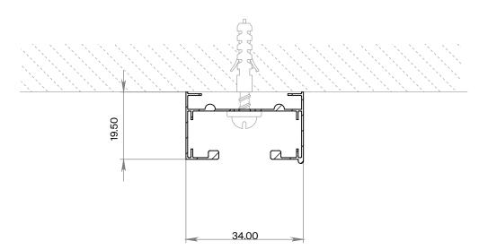
TRACK INSTALLED ON A CONCRETE CEILING
