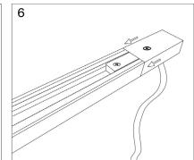
Insert the connected power lead-in into the track. Install the track in the most appropriate way.
