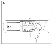
Fasten the phase and neutral conductors on the contact plates using clamping screws.
