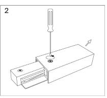
Remove the screw on the front side of the power lead-in using a screwdriver and remove the plastic cover.
