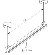
The recommended distance between lamps is 25 cm. The maximum permissible load on the surface-mounted track installed using suspension fasteners is 10 kg per 1 metre.
