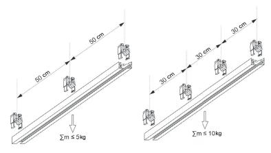
The distance between the holders is selected based on the weight of installed luminaires. The luminaire weight at 1 metre  $\leq$  5 kg -the distance between holders is 50 cm.The luminaire weight at 1 metre  $\leq$ 10 kg – the distance between holders is 30 cm.The recommended distance between luminaires is 25 cm. The max. permissible load on the recessed track installed using holders is 10 kg per 1 metre.
